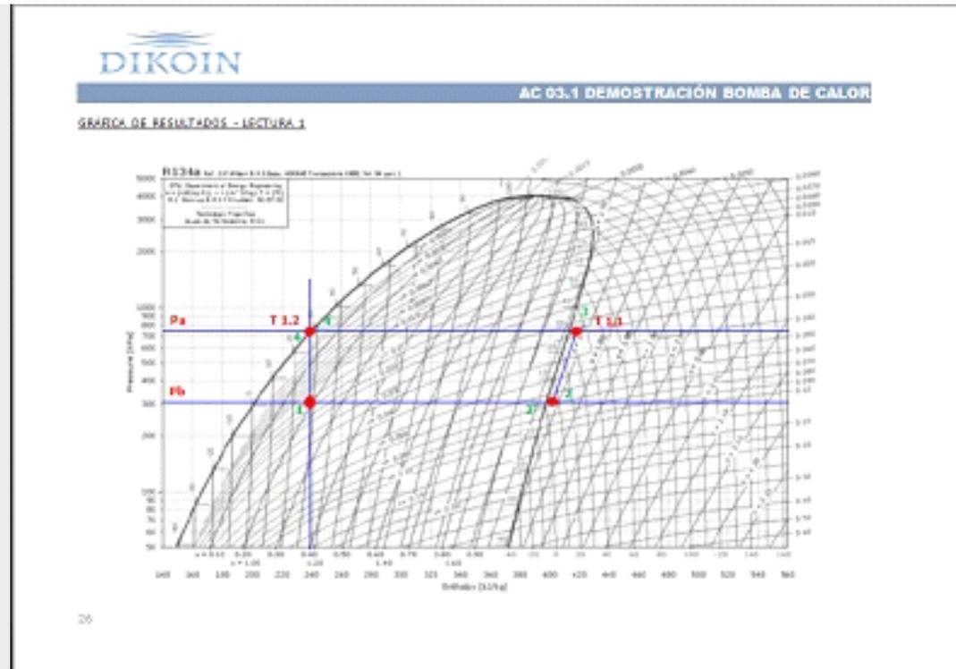
During the experiments, the obtained results are shown in a Mollier Diagram. Pressure-Enthalpy.
