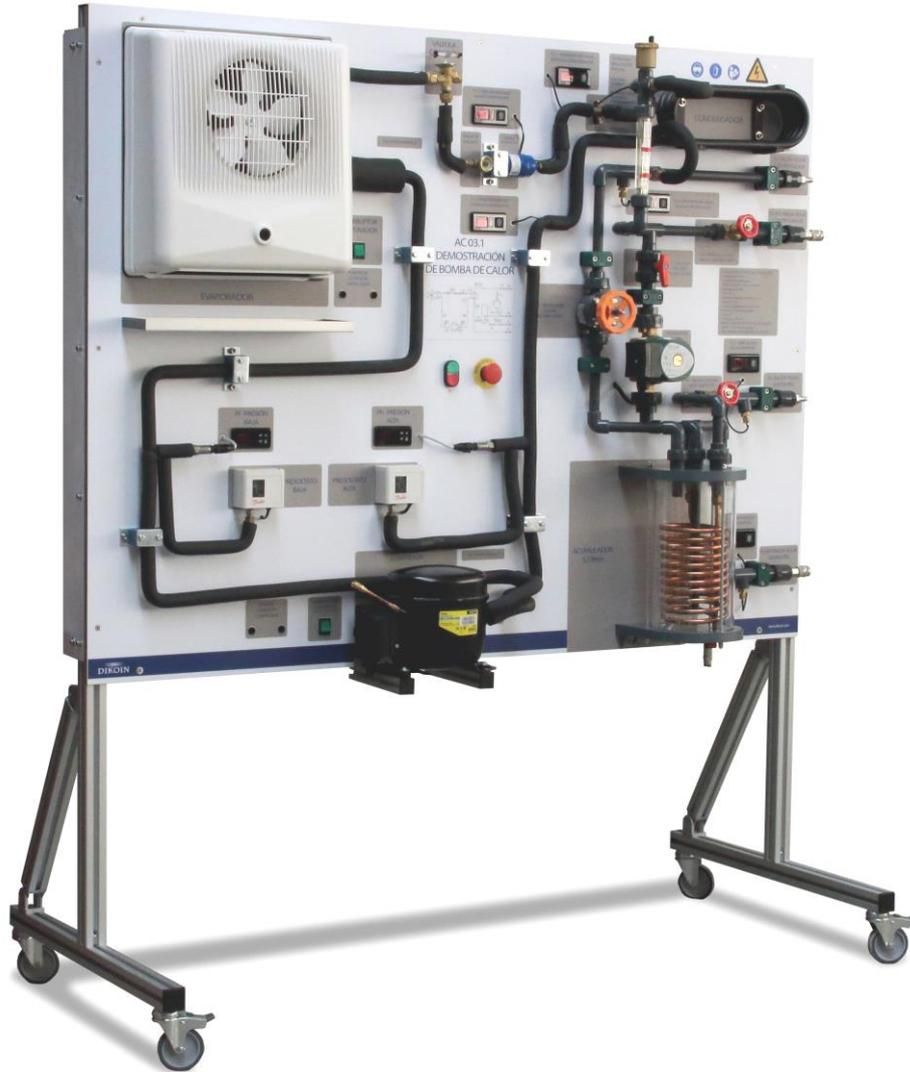
The AC 03.1 equipment demonstrates clearly the operation of a air / water heat pump .
